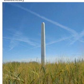
Bladeless Wind Energy (Vortex Bladeless)
